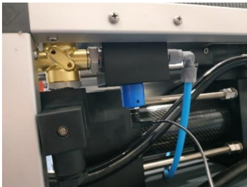
DIVERTING VALVE FIG. 3-11
