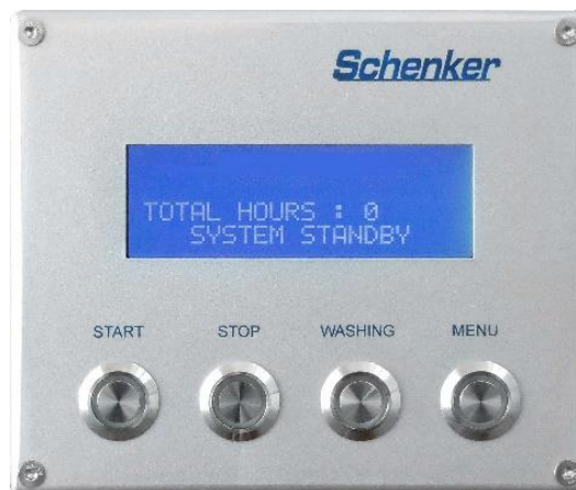
REMOTE CONTROL PANEL FIG. 4-3
